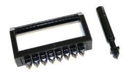
Reagent Plates / Reagent Strips are prefilled with extraction reagents and are sealed with a foil. This foil has to be pierced manually before use, by using the piercing tools (single piercer or 8fold piercer).
