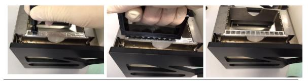
**IMPORTANT** Use single or eightfold piercing tool for opening of <u>all</u> cavities of one row per sample!
