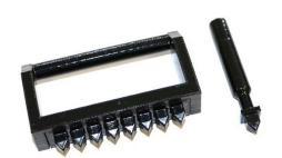
Reagent Plates or Strips are prefilled with extraction reagents and are sealed with a foil. Before use, this foil has to be pierced manually using the piercing tools (single piercer or 8fold piercer).
