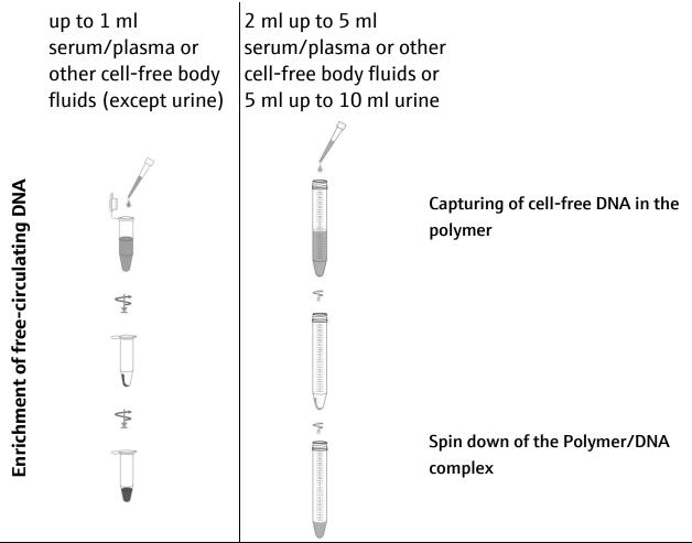
Lysis of the Polymer/DNA complex and sample preparation of freecirculating DNA runs automatically on the InnuPure<sup>®</sup>C16 / C16 touch.
